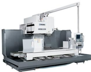
**Pittsburgh, January 29, 2010** – Frontier Steel, a steel service center that distributes and processes carbon steel plate, has expanded its processing capabilities with an OKUMA Millac-1052V heavy-duty, 3-axis vertical machining center. This new piece of equipment increases
